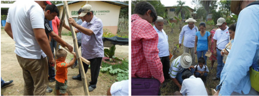
Fig. 3 Calibrating the Level-A, a simple instrument used to trace contour lines on a sloping terrain ( left ), and evaluating soil compaction in the field ( right )
